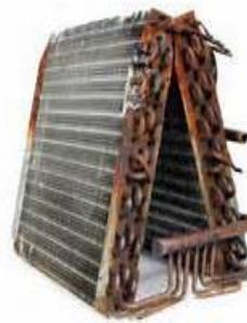
Two conditions necessary to support biological growth are nutrients and moisture. Condensation on the evaporator coils and in the drip pan provides the moisture and particles that bypass the air filter provide the nutrients.
