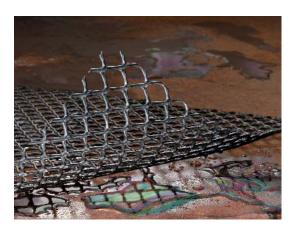
Rigid extruded mesh is manufactured from multiple resins, including polypropylene, polyethylene, polyamides and polyesters. The thickness is 0.100".and have consistent geometric openings of 1/4". This rigid, UV-stabilized net can offer a number of lightweight, high-strength solutions. Used for support, barrier or reinforcement, it is non-corrosive and resistant to most chemicals and oils.
